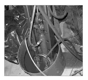
Before. The hose in the middle going to the port is a vent hose, open on the end, to keep dirt and water out.
