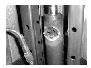
The cylinder showing the burnt-out port and melted piston.
